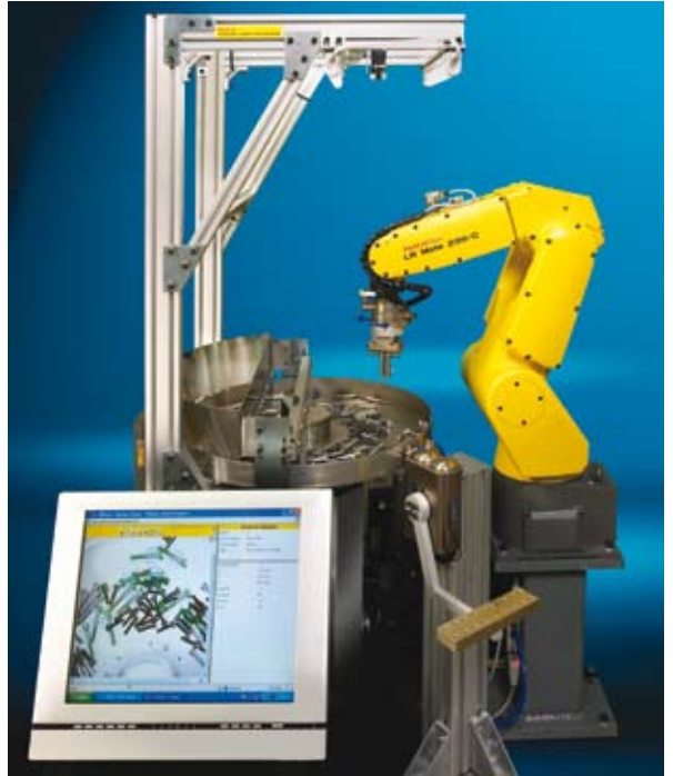
LR Mate 200iC picks & sorts multiple style parts through flexible feeder using built-in iRVision and available Aux. Axis option!
