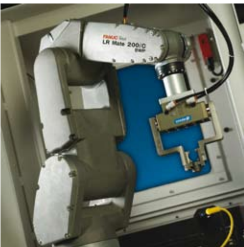
Tough and rugged LR Mate 200iC/5WP used for high pressure washing, deburring and cleaning applications!
