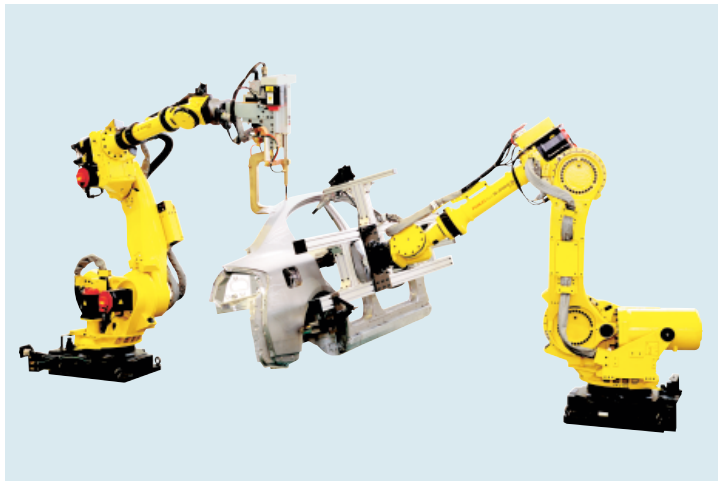
Spot welding by synchronized 2 robots
