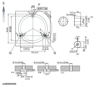
(C)3x common zoneEPosition of the front of the robotF4xM16 depth 30, minimumGGuide bushing (2 pcs)
